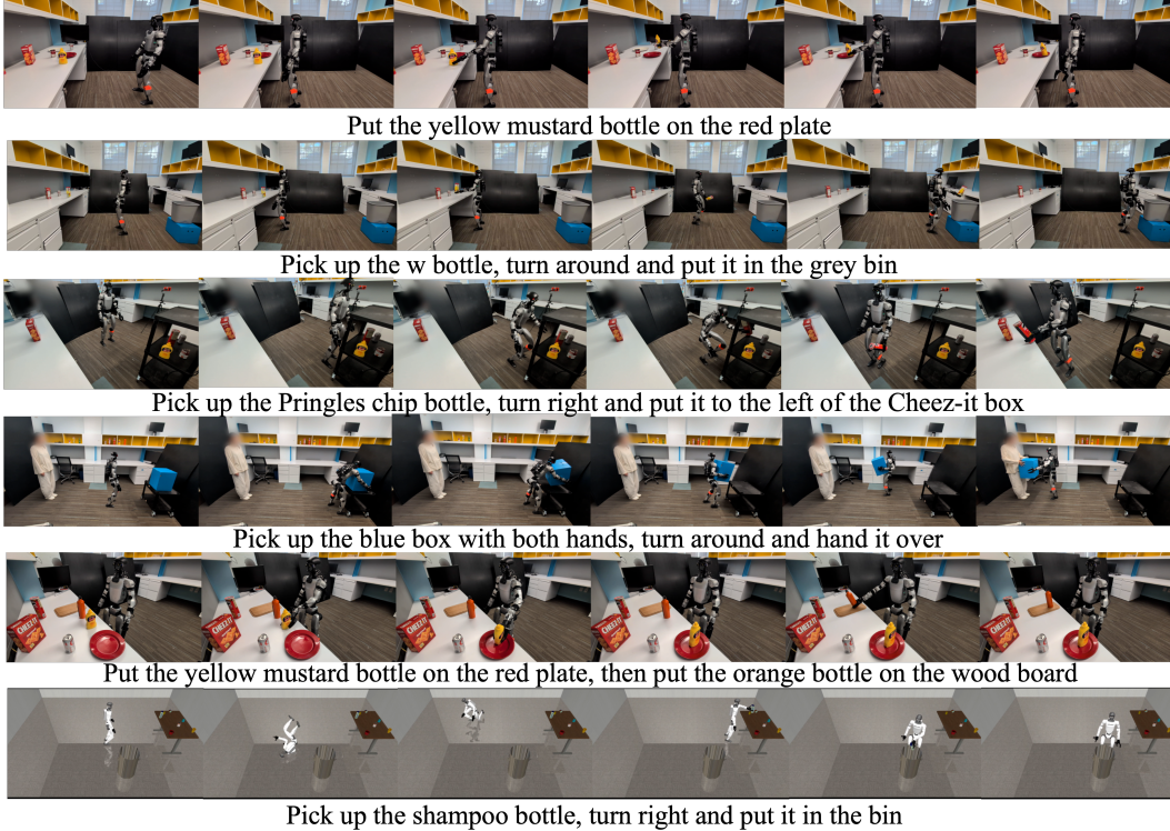
Figure 5: Agentic deployment snapshots with VLM text prompt. The same 10-D controller, driven by the agentic planner, executing a range of loco-manipulation tasks on the Unitree G1 hardware and in simulation: pick-and-place, pick-transport-place, squat-pick, bimanual-pick-and-hand-off, bilateral pick-and-place, and task continuation after fall recovery. No controller-side change, data collection or model fine-tuning is required between tasks.
