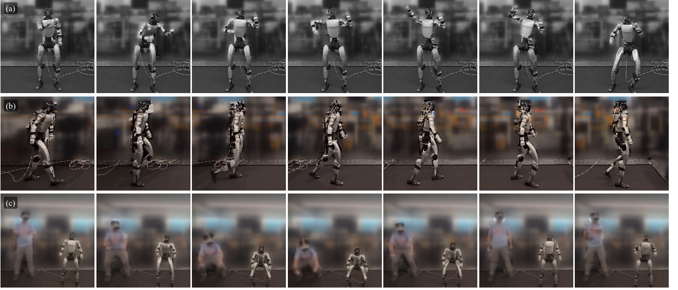
Figure 5. MorphMimic on a real Unitree G1. (a) Dance, (b) walking, and (c) teleoperation, in which the robot follows a human operator. Frames run from left to right at intervals of 1.0 s in (a), 0.5 s in (b), and 2.0 s in (c).
